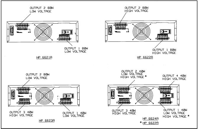
Figure 4-1. Output Connections
